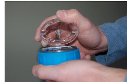
If there are batteries already in the probe, remove them by forcing your thumb under the mid-section of the battery while pushing up.
