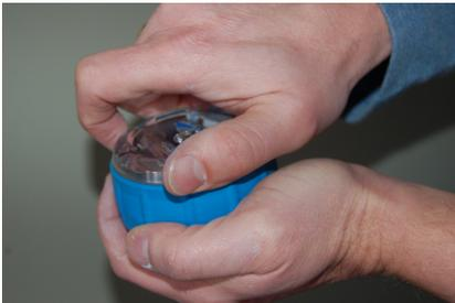
normal. As the cover loosens the bumping will stop and the cover will turn freely. Spin the cover free. *(The screw in the center of the cover will remain with the cover as it is removed. Do not remove the cover by unthreading the screw unless the battery cover is seized and you cannot loosen it by hand. If the screw should come loose or if you unscrewed it,*
